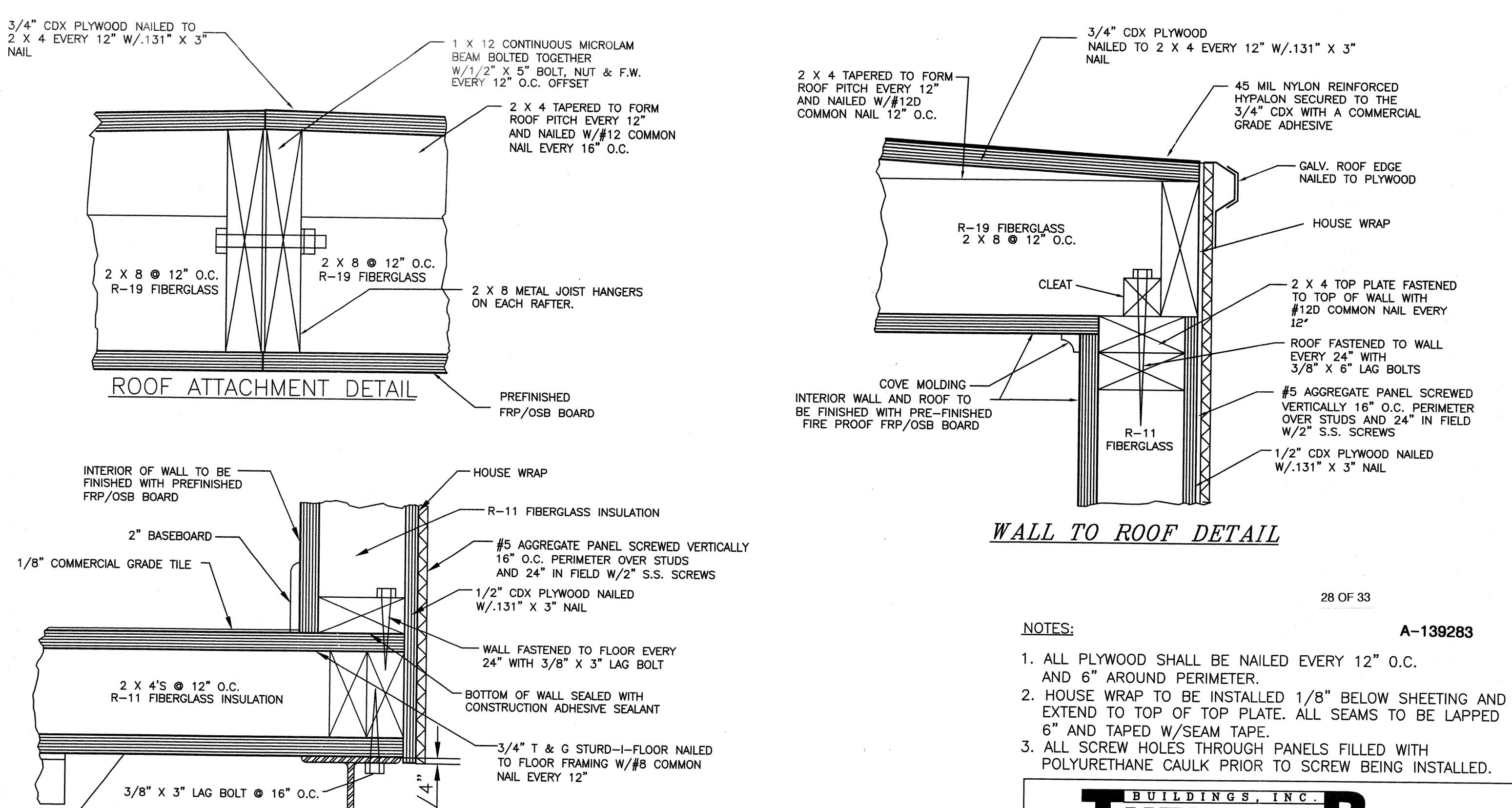
BOTTOM OF FLOOR IS 3/4" CDX PLYWOOD SEALING WITH AN ASPHALT UNDERCOATING
