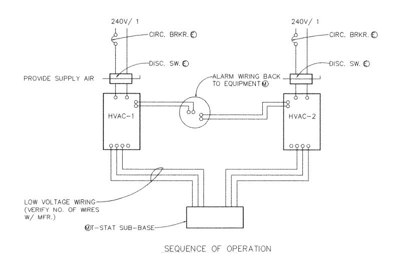
AN ENVIRONMENTAL CONTROL PANEL, HOFFMAN CONTROL ENCLOSURE A16148CHQRFG, BACK PANEL A16P14, SHALL OPERATE HVAC-1 AND HVAC-2. THE CONTROL PANEL WILL ALTERNATE THE OPERATION OF HVAC-1 AND HVAC-2 FOR EQUAL PERIODS OF TIME. BUT, SHOULD THE COOLING LOAD REQUIRE THE OPERATION OF BOTH HVAC-1 AND HVAC-2, THE CONTROL PANEL WILL OPERATE BOTH UNITS SIMULTANEOUSLY.
